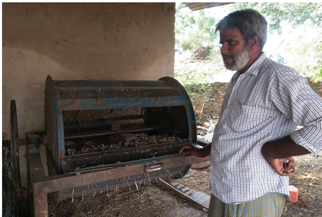
Semi processing of Acorus calamus rhizomes by using polishing machine
